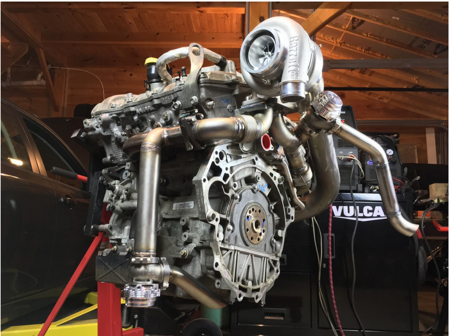
Saab 9-3 2.8T V6 fabrication - 750 hp capable Garrett GTX3076R gen2 turbo system with dual Tial 39mm external wastegates and screamer pipes
