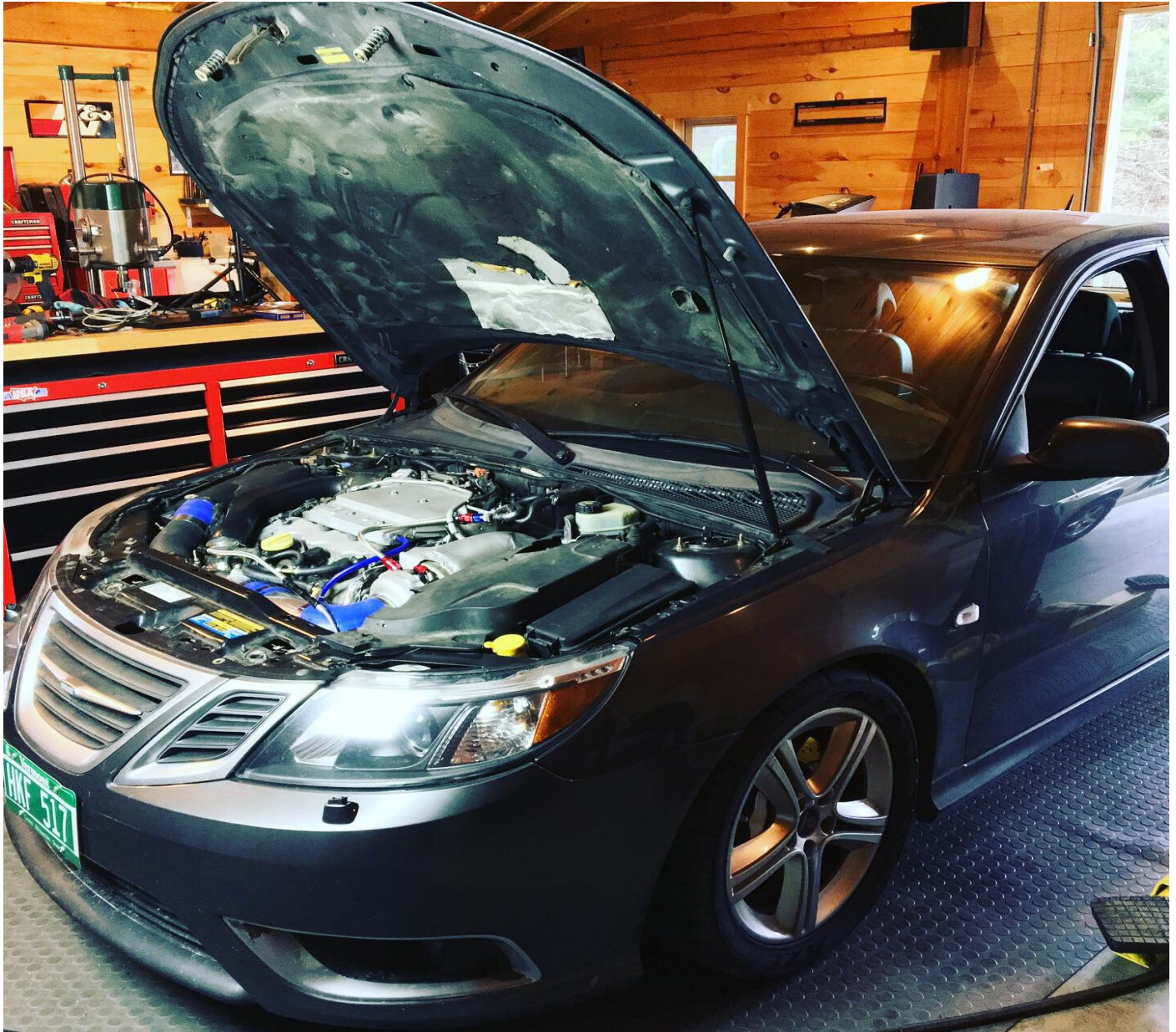
Vermont Tuning shop interior and my personal 2009 Saab 9-3 Aero XWD fitted with a Garret GTX3076R gen2 turbo running on E85.
