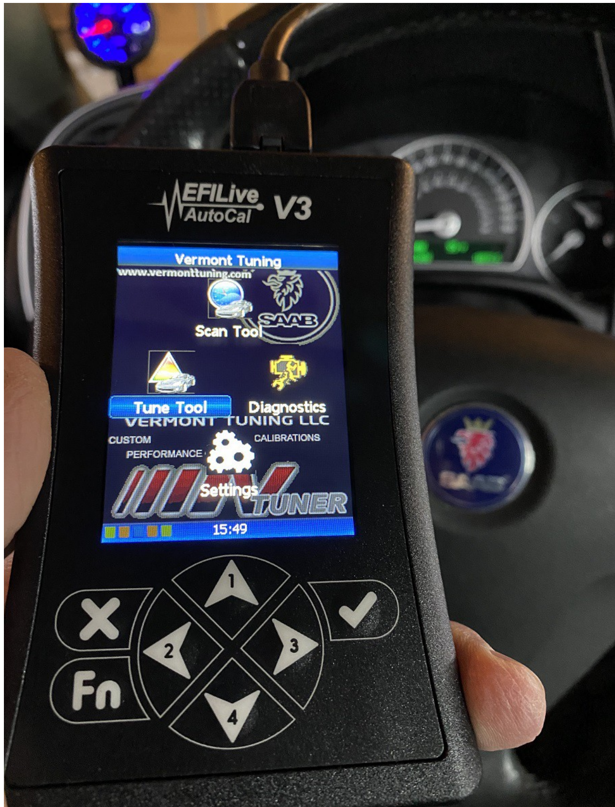
Handheld tuning system used to program engine calibration software, record high speed data logs and provide diagnostics
