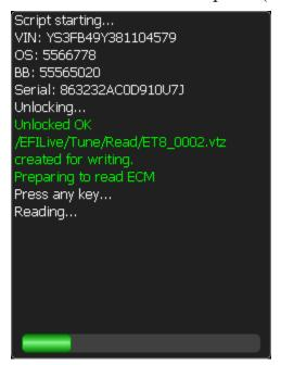
The display will show a progress bar and will prompt you to turn the key to the "Off" position when it is finished (The T8 read procedure takes  $\sim 15$  minutes to complete).
