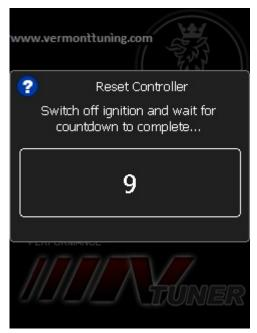
After turning the key to OFF, press the "**Ok**" button and it will run a count-down timer to allow the computer in the car to reset before you start the engine. Remove the key from the ignition momentarily.
