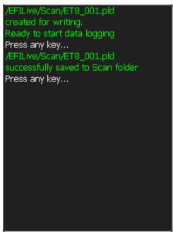
I like to see 5-10 minutes of mixed driving with some wide open throttle acceleration through the first couple of gears. To transfer the logs from the handheld to your computer, start the EFILive V8 Explorer application and click on the "Scan" folder. Your data logs will appear under this folder with file names like ET8\_0001.efi.
